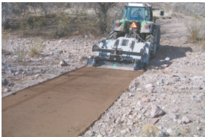
Italian-made machine can crush rock, stone, concrete and cement up to 20 in. in dia. An adjustable breaker bar controls size of material being produced.
