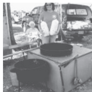
Home-built, gas-fired "butcher kettle" corn popper is built around a pair of 2-ft. dia., cast iron hot butchering kettles.
