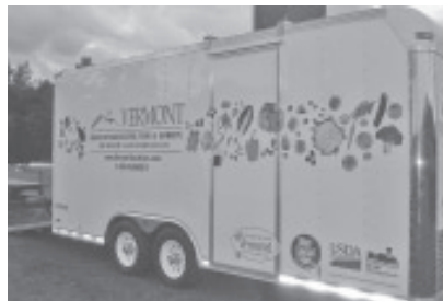
Developed for Vermont fresh berry producers, this mobile freezer preserves fruit in the field. Trailer is equipped with a 5 hp, single-phase compressor and a fruit drying station.
