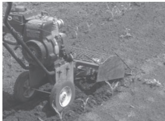
Ostendorf fitted his rototiller with skis, side shields, and a protective cover over the tines.
