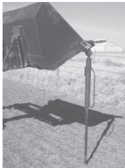
Zweifel's T-post driver hangs from the front edge of loader bucket.
