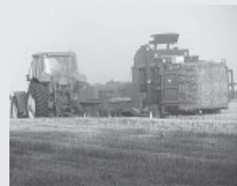
**Machine wraps groups of bales tightly with steel bands and then ejects the bundle on-the-go.**
