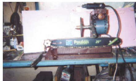
Chainsaw bar bolts to wooden frame. A knob at one end of the bar is used to advance the chain.
