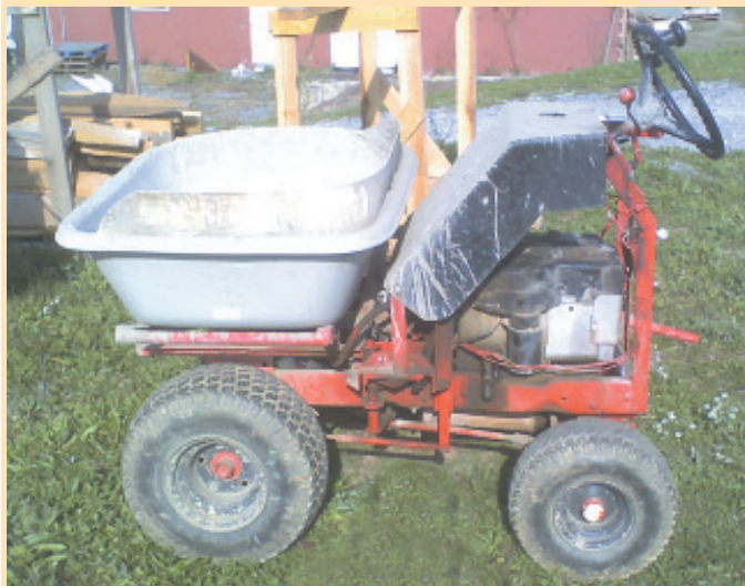
Self-propelled "concrete buggy" was made by cutting down the frame of a Deere hydrostatic riding mower and mounting a wheelbarrow tub over the drive wheels.
