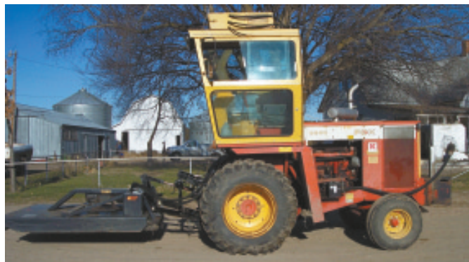
"It's like having a giant lawn mower with the deck out in front of me," says Junior Schneider, who converted a SPFox silage chopper to cut brush and small trees.
