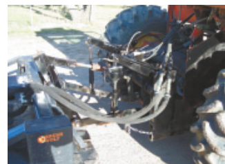
Schneider designed mounting brackets to attach brush cutter to front of chopper.
