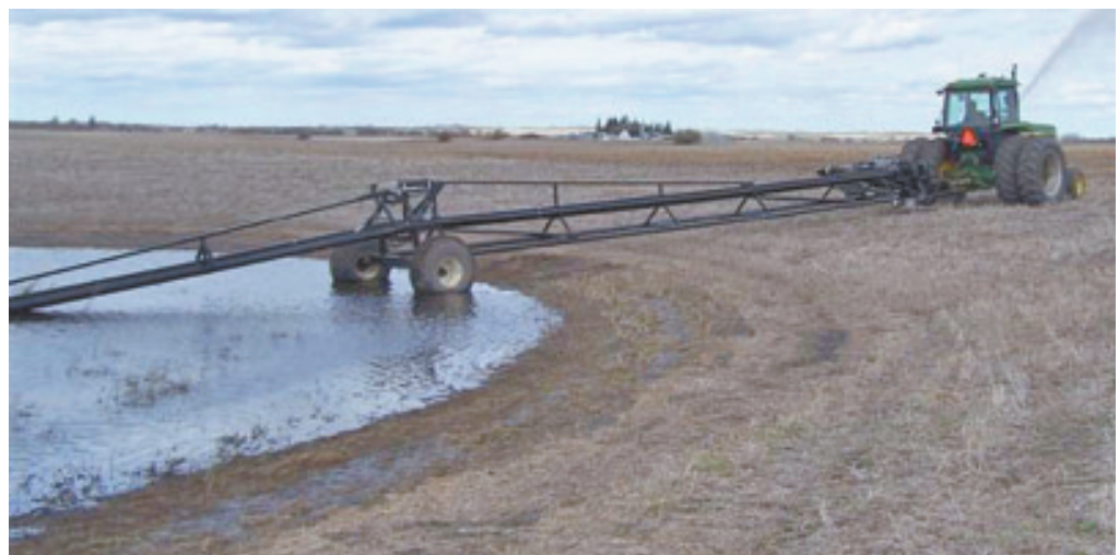
Water cannon is often used to pump water out of low spots before planting. Note blast of water shooting out at front of tractor.
