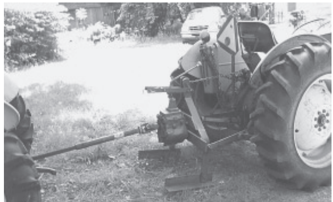
Larry Randall uses a 4-speed truck transmission to start a dead tractor through its pto shaft. He welded a GM pickup transmission to a 3-pt. hitch frame.
