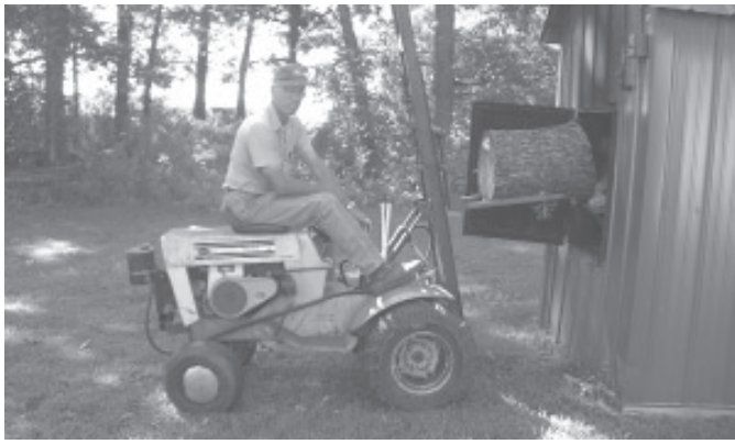
James Bachert converted his 1969 12 hp Sears garden tractor into a handy forklift, attaching a home-built mast to the rear end.
