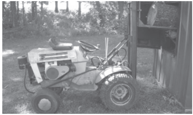
He installed the seat on the hood of the tractor and replaced the hydrostatic hand control with a double action pedal.
