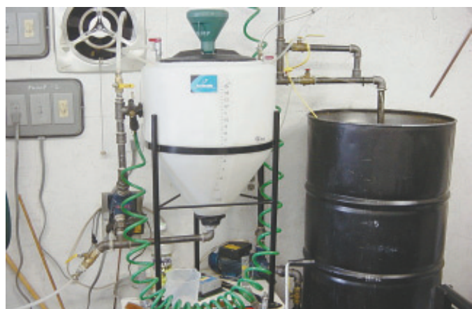
Steve Veenstra developed his cold evaporation process to reduce the amount of time he had to put into making biodiesel.
