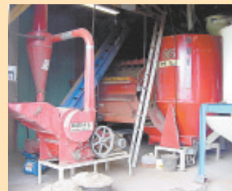
The Siedschlags recently set up a farm-sized pellet plant in their shop which includes a tub grinder, hammer mill, screener, and self-unloading wagons. Their goal is to automatically make 800 to 1,000 lbs. of pellets per hour.
