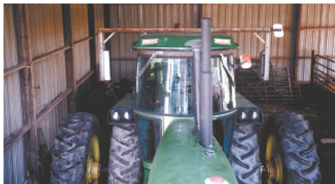
Mirrors are bolted to a length of angle iron that extends across top of tractor cab.
