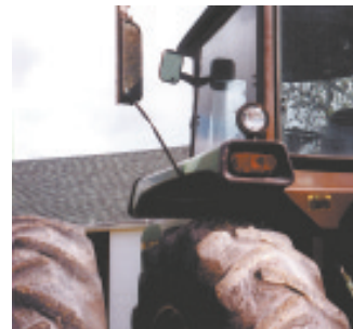
By mounting a pair of big truck mirrors on his Deere 4640, Jerry Allen can see around wagons and wide equipment.
