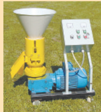
Pellets shown above were made by Tiger Tec's 7 1/2 hp. pellet mill (right). It's geared down to run slower and has more torque than other similar-size pelletizers.
