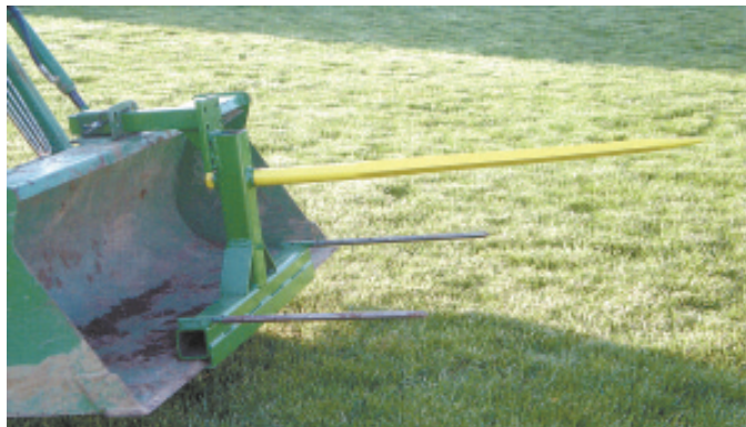
Bale spear fits into 2-in. receiver hitch welded to top of bucket.
