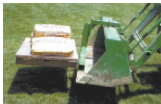
The two small lower spears allow unit to also be used as a pallet mover.
