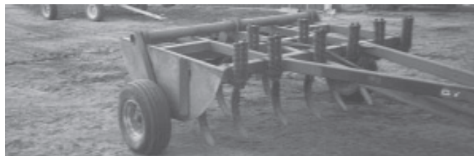
Louis Smith removed chisel plow's back row of shanks and mounted some of them between the plow's front row of shanks (above). He welded a 24-in. high sheet of steel on back and also welded a "half moon" onto each side of the plow frame to form a box.
