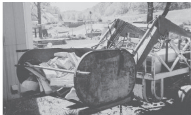
Art Freymiller converted a 250-gal. oil tank into this big loader bucket. It holds about a 1/3 face cord of wood.
