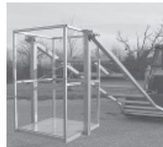
Self-leveling "basket" swivels on a pair of steel pins and is kept level by a metal rod.
