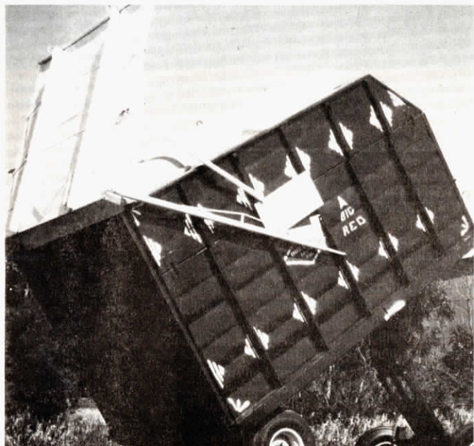
Dohrman self-opening endgates can be adapted to other makes of silage wagons.
