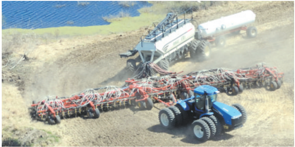
Bourgault’s 6000 Series Air Seeder is available with tank capacities up to 700 bu. Photo shows it towed behind a 75-ft. toolbar
