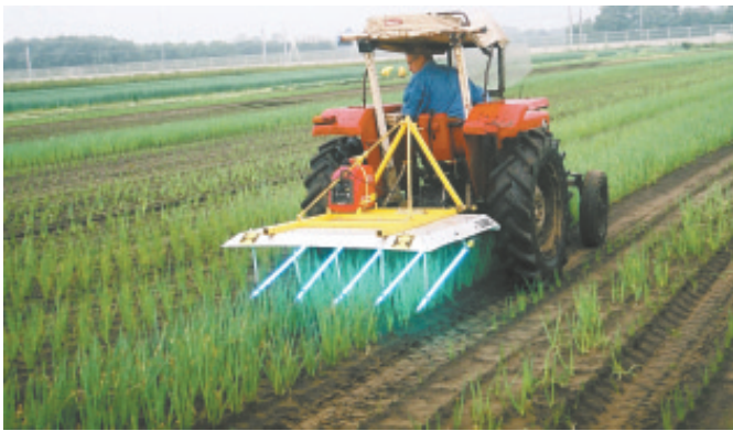
Ultraviolet light bulbs are passed over plants to kill crop diseases. An on-board generator provides the electricity.
