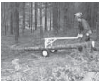
Although it weighs just 57 lbs., log mover can move up to 15 times its own weight.
