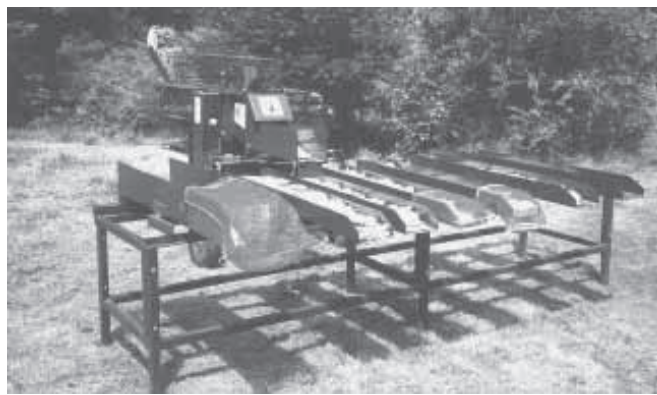
Hydraulically powered "Kindla" makes 100 bags of kindling in an hour. Bags sell for $5 or more apiece.
