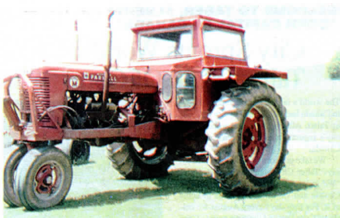
Home-built cab has a heater, defroster, windshield wipers, and a radio.
