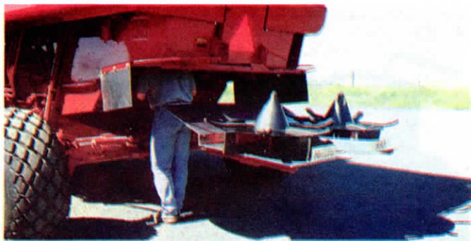
Once installed, straw spreader cones mount on new chaff spreader and entire unit slides out for easy access to sieve area.
