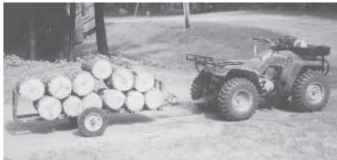
Trailer is narrow enough to wind through the woods with a load of up to 600 lbs.
