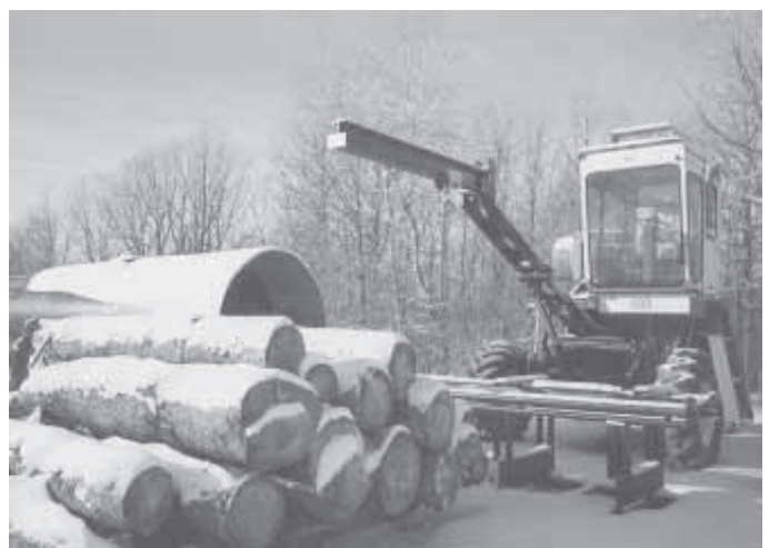
Crane boom is made from I-beams powered by combine hydraulics.
