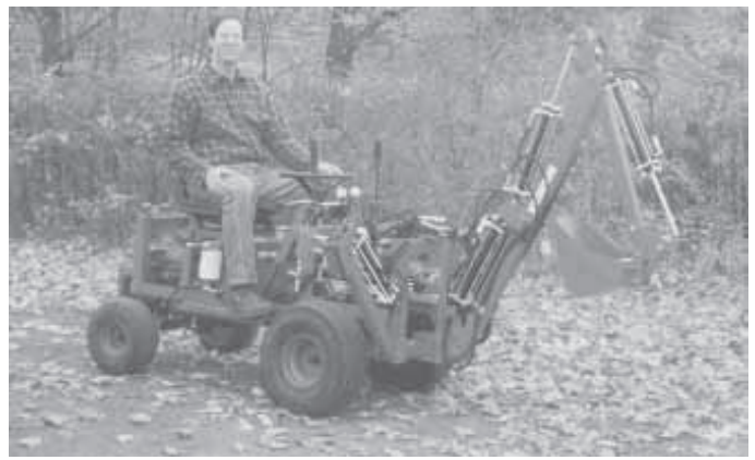
Vincek made the tractor’s hydraulic cylinders out of shock absorbers.
