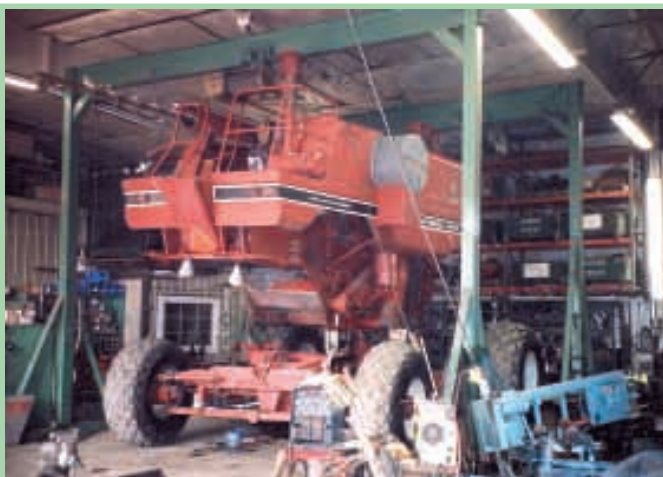
J & M Fabrication mounted the body of a 1998 Case IH 2166 Axial Flow combine on the wheels, axles, and frame of a 1980 Case IH 1470. Here the body of the 1470 is being lifted off its frame.
