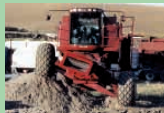
J & M Fabrication mounted the body of a 1998 Case IH 2166 Axial Flow combine on the wheels, axles, and frame of a 1980 Case IH 1470. Here the body of the 1470 is being lifted off its frame.
