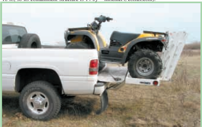
Pickup-mounted ramp is strong enough to load the biggest ATVs. It'll also carry the back end on road trips.
