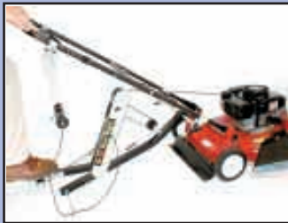
To start mower you simply turn a crank on mower handle and then step on pedal.
