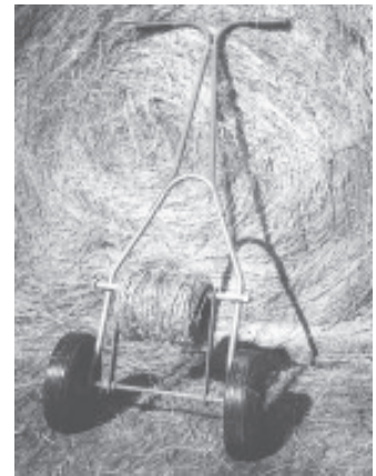
Barbed wire unroller carries roll off the ground to keep wire from tangling.
