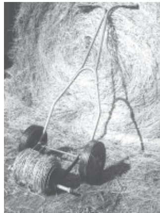
Barbed wire unroller carries roll off the ground to keep wire from tangling.
