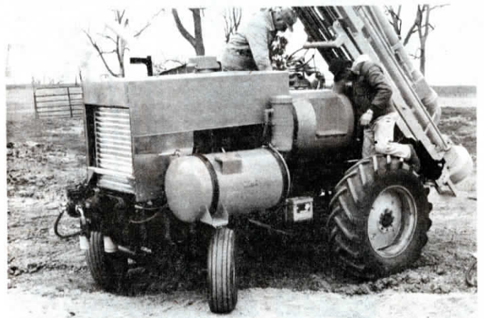
The power unit is equipped with a revamped Clark forklift mast which raises and lowers a heavy-duty manure prop and pump to empty out pits.
