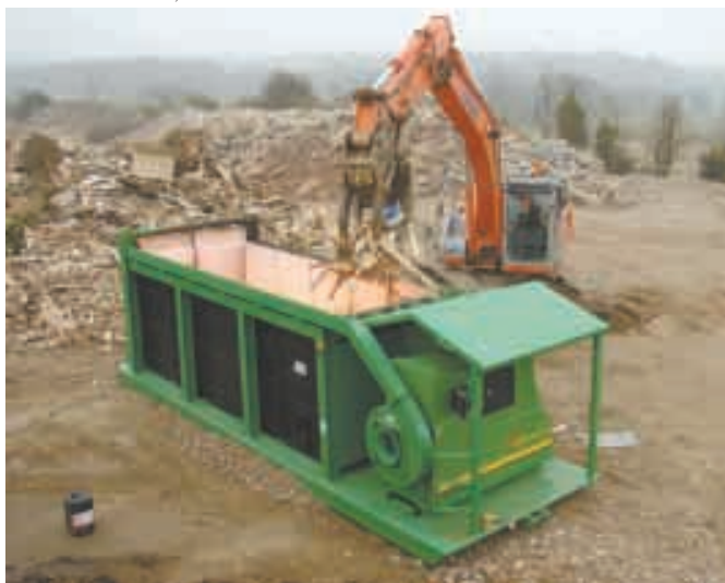
Burn box can handle timber residue, stumps, construction waste, and other debris. High velocity airflow creates an invisible curtain over fire and rotational turbulence within it.
