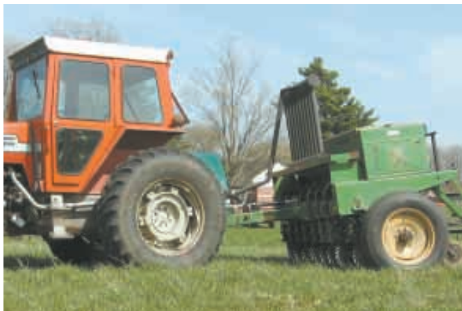
With the help of his school's auto class, vo-ag teacher Ray Morrison designed a manifold large enough to handle his tractor's exhaust and mounted it on his grain drill.
