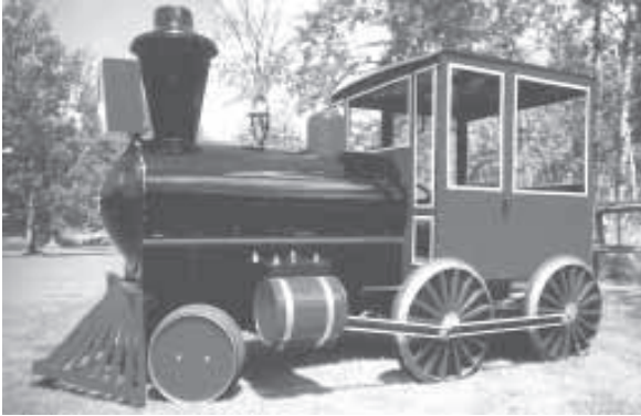
Ray Seefeldt's 8-ft. long locomotive was built over a Ford 25 hp, hydrostatic 2-WD garden tractor.
