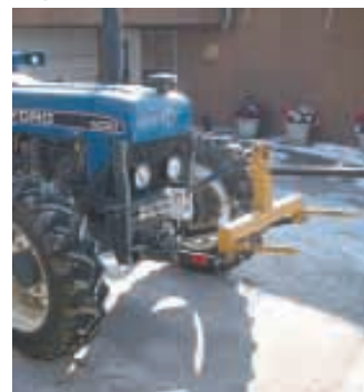
Lyndon Dunbar's home-built front hitch folds out of the way when not in use.
