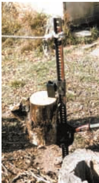
Steel wedge is designed to bolt onto a conventional hi-lift jack, turning it into an effective low-cost log splitter.
