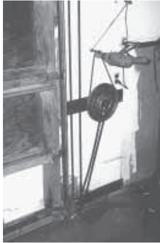
Reversible drill works with pulley system to open and close Fred Davison's 16 by 12-ft. wooden door.
