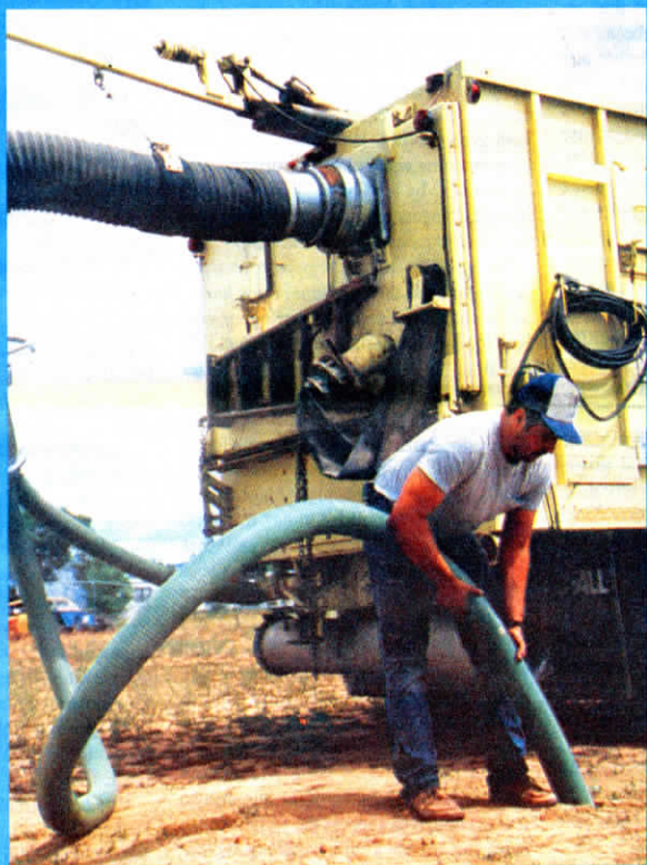
Operators slip hoses down tunnels to suck rodents out “alive and kicking”. Main hose has enough suction to pick up a bowling ball.
