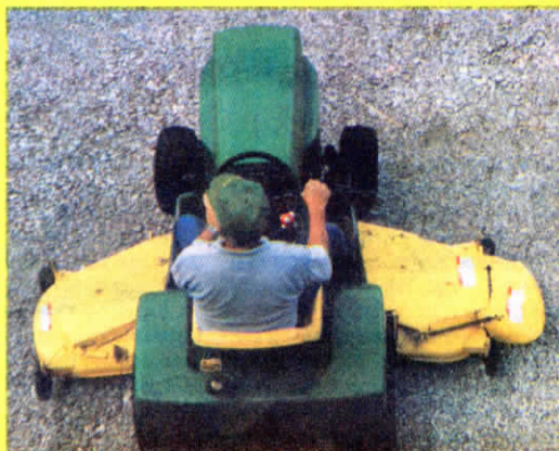
Moss's double deck Deere looks like a factory-built model. Photo below shows how he added two 18-in. wings and double pulleys operated by a central drive. (Editor's Note: See pages 26 - 28 for an "Owner's Report" on riding lawn mowers.)
