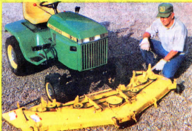
Moss's double deck Deere looks like a factory-built model. Photo below shows how he added two 18-in. wings and double pulleys operated by a central drive. (Editor's Note: See pages 26 - 28 for an "Owner's Report" on riding lawn mowers.)
