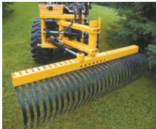
A system of hydraulic cylinders, combined with tractor's 3-pt. and hydraulic top link, let Gerken lift, lower, angle the rake left and right and change the pitch.
