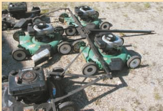
Don Kuntz ganged five push mowers together in such a way that they flex over ditches and other uneven terrain.
