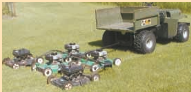
Don Kuntz ganged five push mowers together in such a way that they flex over ditches and other uneven terrain.
