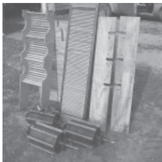
Different screens are available for threshing a variety of grains.
