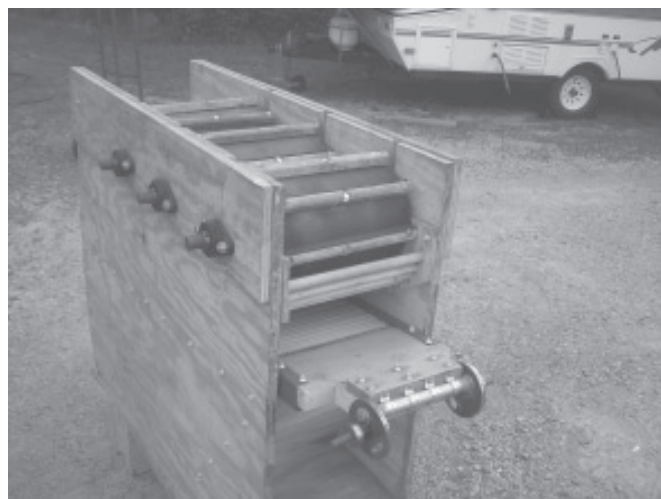
Latest version of mini thresher is powered by a 5 hp gas engine.
