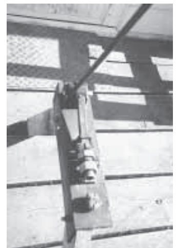
Pushing down on handle cracks nut against a 2-in. bolt.
