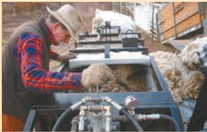
James Lunders designed this trailer-mounted wool press to help offset low wool prices and high fuel prices.
