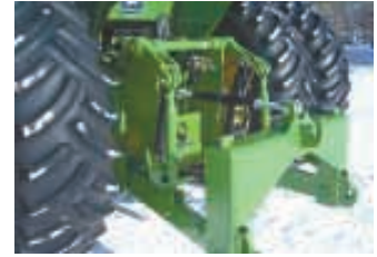
Mandako also makes Cat. III hitches, such as this one mounted on a Deere 4630.
