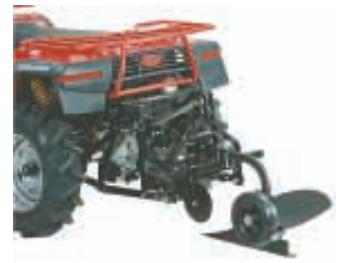
Hitch hooks up to company's plow, disk, harrow, furrower, cultivator, rake and rear blade.
