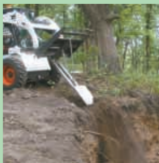
The 20 by 18-in. spade works great for digging trenches when attached to skid loader forks.
