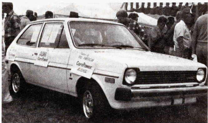
ADM's re-manufactured Ford Fiesta. The company has also modified an Oldsmobile diesel to run on 10% alcohol.
