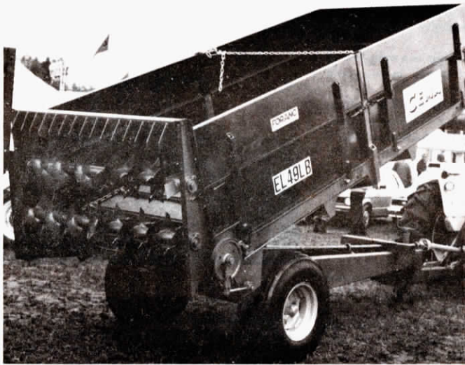
With sides and rear beaters, the 7-in-1 wagon is equipped as a dumping manure spreader.
