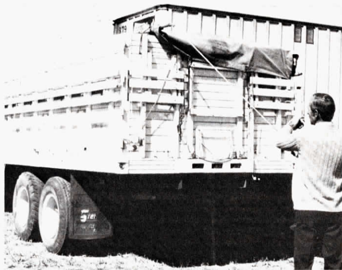
Several turns of the long crank unrolls the tarp. It's pulled via a rope to re-cover the load.
