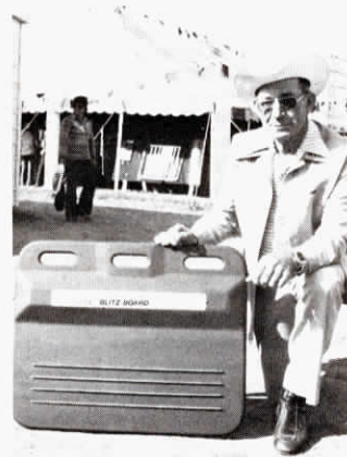
Robert Jones, pictured, says the Blitz Board combines the best of an electric prod and a plywood sorting panel. Center hand grip section is equipped with a trigger for turning shocking device on or off.
