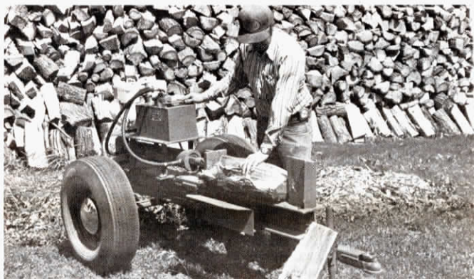
Self-powered Schweiss Wood Splitter splits wood with nearly 38,000 lbs. push at 3,000 psi. Tractor-powered model also available. Can crusher attachment is optional.
