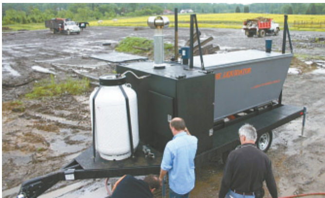
Carcass disposal unit uses alkali hydrolysis to convert animal carcasses into liquid.
