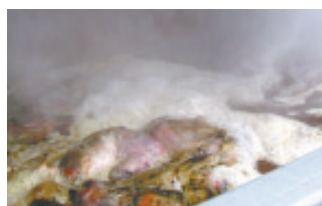
Two hours into the cycle, chickens are being digested rapidly with feathers virtually gone (left). Digestion is virtually complete in 16 hours. Note liquid soap floating on surface (right).
