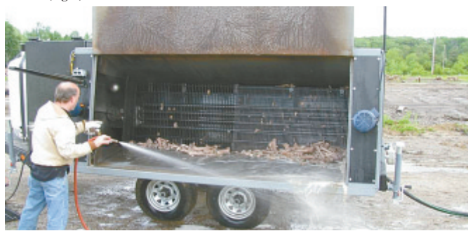
Tipped into cleaning position, the unit can be easily hosed out. A few bone fragments are the only solids left.
