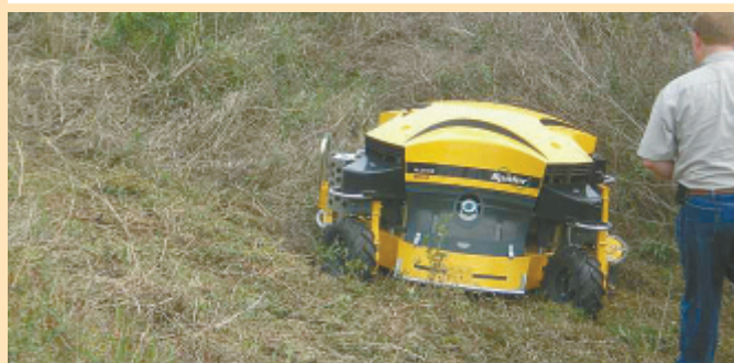
Radio-controlled mower can go on uneven terrain too dangerous for human operators.
