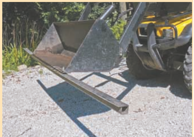
Cutterbar consists of an 8-ft. length of 1 1/4-in. sq. steel tubing with a length of 2-in. wide, 1/4-in. steel strap ground down to a cutting edge.
