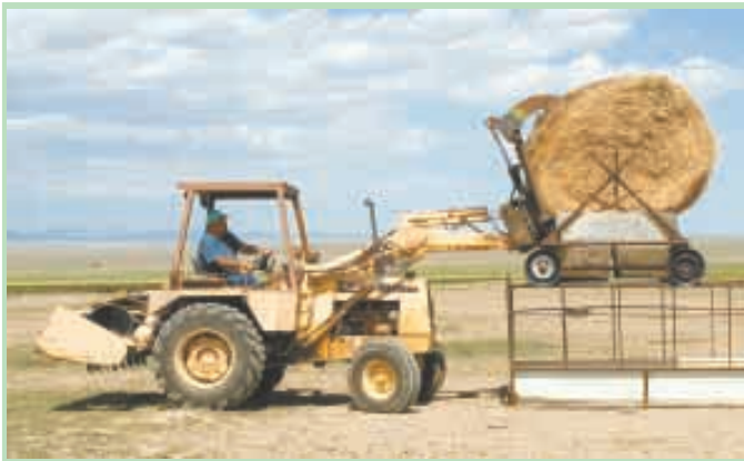
Frank Thompson built this 32-ft. long feed bunk with an unrolling cart on top that makes it easy to spread out a big bale.
