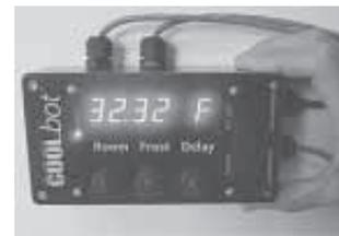
CoolBot lets you use an air conditioner to keep produce fresh. A micro-controller constantly monitors the walk-in cooler temperature.
