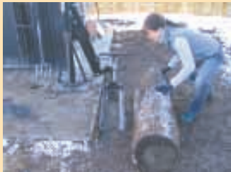
Operator rolls log onto a loading cradle (above left) and cranks a handle to raise cradle (above right), then winches the wood to the proper height and guides it through the furnace door.
