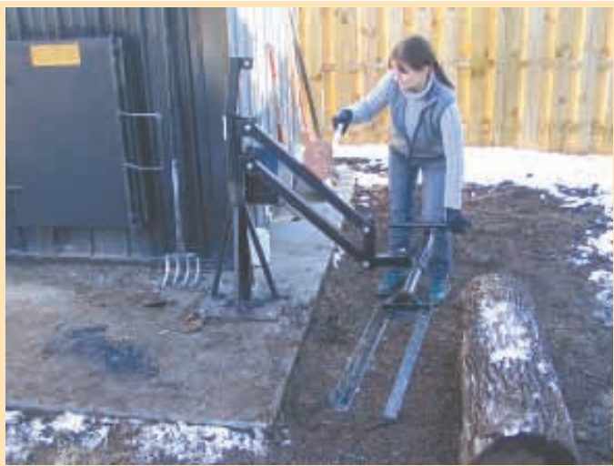
Hall Log Loader is designed to pick up a big chunk of wood and feed it into a stove.
