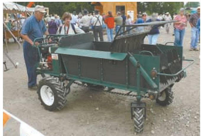
Paul Shetler’s 25-bu. self-propelled manure spreader eliminates the need for a tractor.
