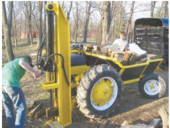
There's a 7-ft. long splitter beam assembly on back built out of an 8 by 8-in. H-beam. Wood is split with the splitter in the vertical position.
