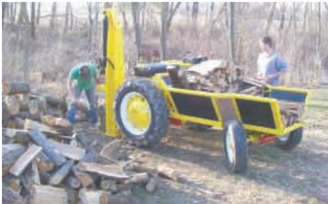
Self-propelled log splitter is built around the back end of a 1949 Allis Chalmers tractor.
