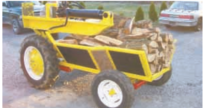
When splitter isn't in use it drops hydraulically into a horizontal position for storage.
