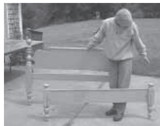
Headboard serves as back of bench and provides the rear legs, while the footboard provides the front legs.
