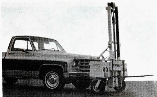
Hydraulic, self-contained pickup forklift can lift and lower 1,500 lbs. 230 times without recharging its built-in batteries.
