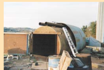
The firebox is a 5,000-gal. fuel tank, surrounded by a 30-ton feed bin.
