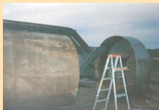
The firebox is a 5,000-gal. fuel tank, surrounded by a 30-ton feed bin.
