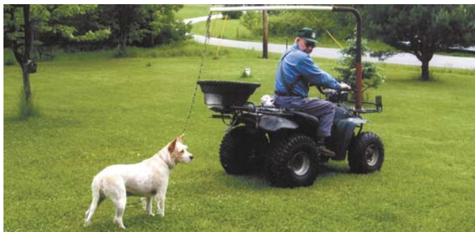
Larry Flaharty made this "dog walker" for his 4-wheeler. "The boom allows the dog to run around the 4-wheeler without getting in contact with it," he says.
