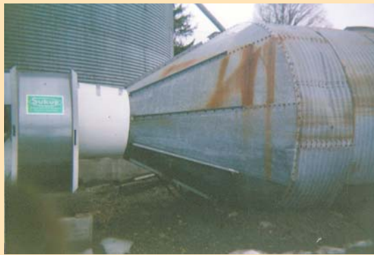
Last year Oliver Place used a wood-burning corn dryer for about half of his 50,000-bu. corn harvest.
