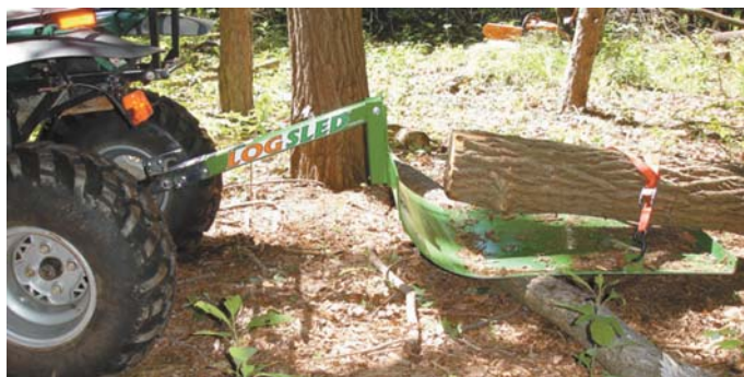
Steel sled can be pulled by an ATV. It lets you skid big logs without digging into the ground.
