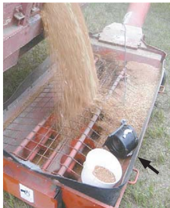
Fan blows away dust as grain is unloaded into auger.
