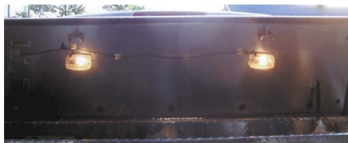
Lights mount inside Chapman's pickup bed-mounted toolbox. He turns the lights on or off by flipping a switch near toolbox's latch.
