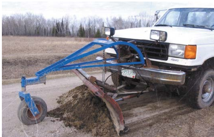
Arched steel frame is supported by a 10-in. caster wheel. It eliminates the washboard effect you normally get with pickup-mounted blades, says inventor Richard Hauner.
