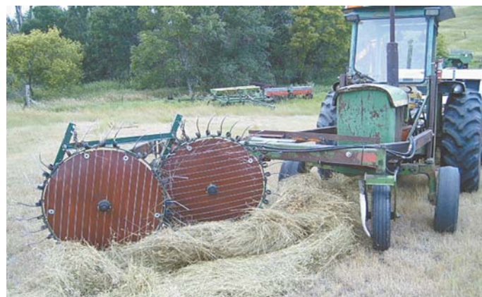
Egli's front-mounted rake can be swung left or right, and also flexes up and down.
