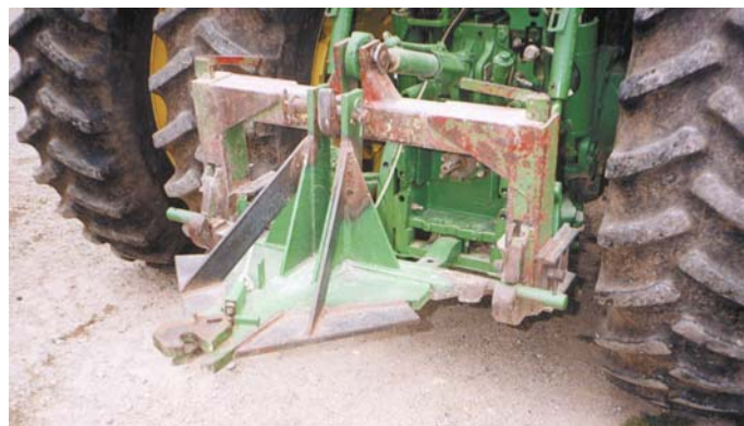
Self-aligning 3-pt. hitch is equipped with a 1-in. thick steel guide, and a locking mechanism that automatically locks into the drawpin in the implement's tongue.
