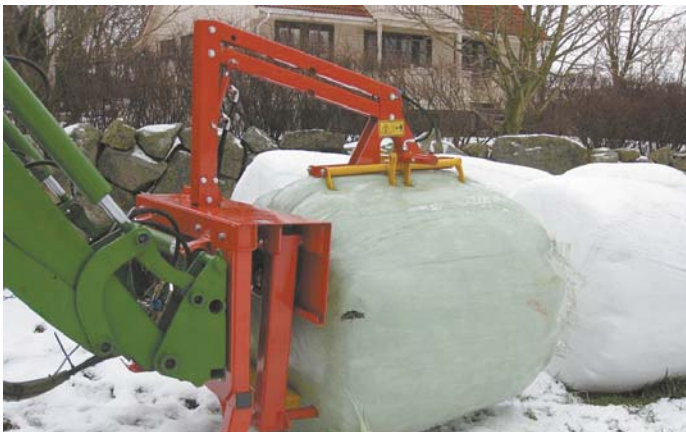
Bale Stripper stabs bale with top lift arm and in the side with moveable spears.
