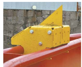
Plastic-cutting knife bolts to rim of TMR mixer. It slices through bottom of bale.
