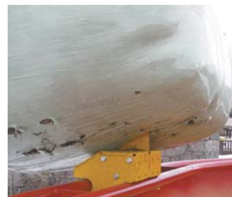
Plastic-cutting knife bolts to rim of TMR mixer. It slices through bottom of bale.
