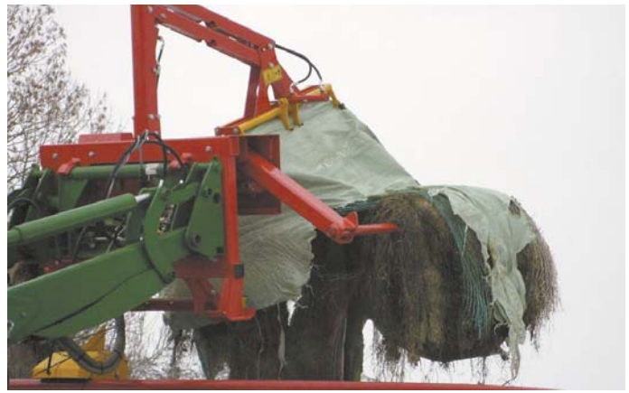
Arm pulls bale out of plastic once it's split on the bottom. Handles up to 5-ft. bales.
