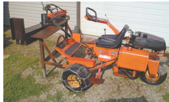
Shawn Smith built this zero-turn log splitter out of an old Toro greens mower.
