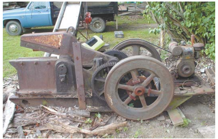
Machine is equipped with a pair of 4-in. wide flywheels. An old hay elevator is used to carry wood chunks away.
