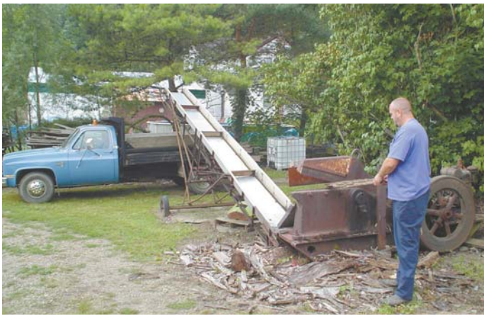
Built originally to crunch through 1/4-in. steel plate or 1 1/2-in. round stock, Shawn Smith's alligator-style wood shears cuts through wood with ease.
