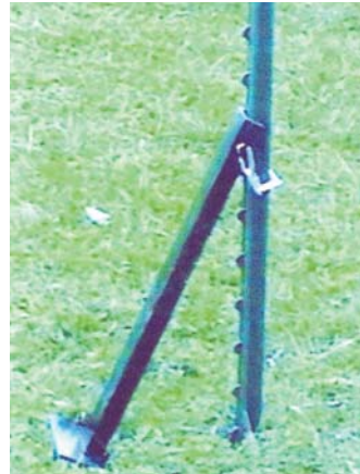
Quik T-Post Puller uses leverage from a catch plate to push post up.
