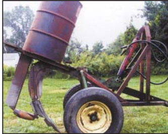
A 55-gal. barrel feeds rock down through a trough and into a 4-in. dia. "bullet" mounted behind subsoiler's single shank.
