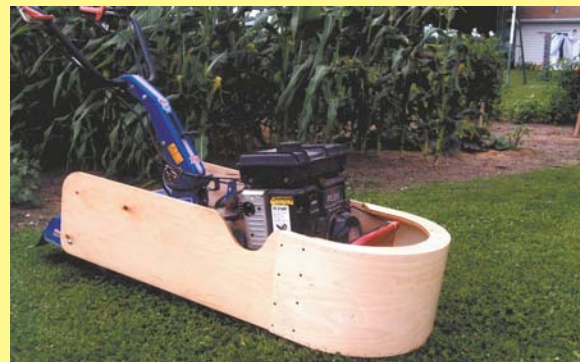
Castor wheel under front end follows garden terrain. Shroud can be removed quickly by pulling two bolts.
