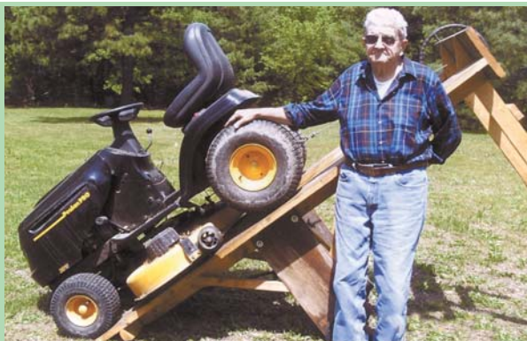
Once tractor reaches the balance point, the lift slowly tilts back down until all four legs are on the ground.
