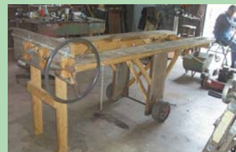
An 18-in. dia. steering wheel at back end of lift serves as a winch. It's attached to a 3/4-in. dia. shaft.
