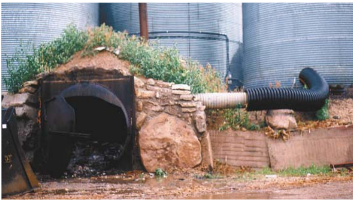
Home-built corn stalk bale burner pre-heats air for Ries's crop dryer. A length of plastic tubing runs to base of wet grain holding bin.
